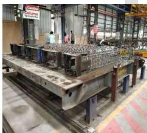
Figure 5. Reinforcement with notch plate
