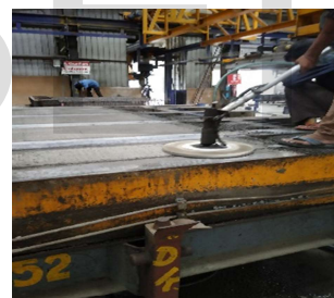
Figure 7. Finishing with floater machine
